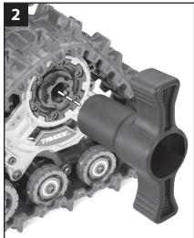
Remove the stub axle nuts from the Traxx drive units using the included 17mm wheel wrench.
